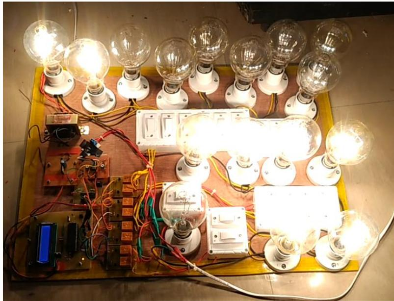
**Fig. 4** Showing normal condition i.e. the load is within the set limit so that all load remains ON.
